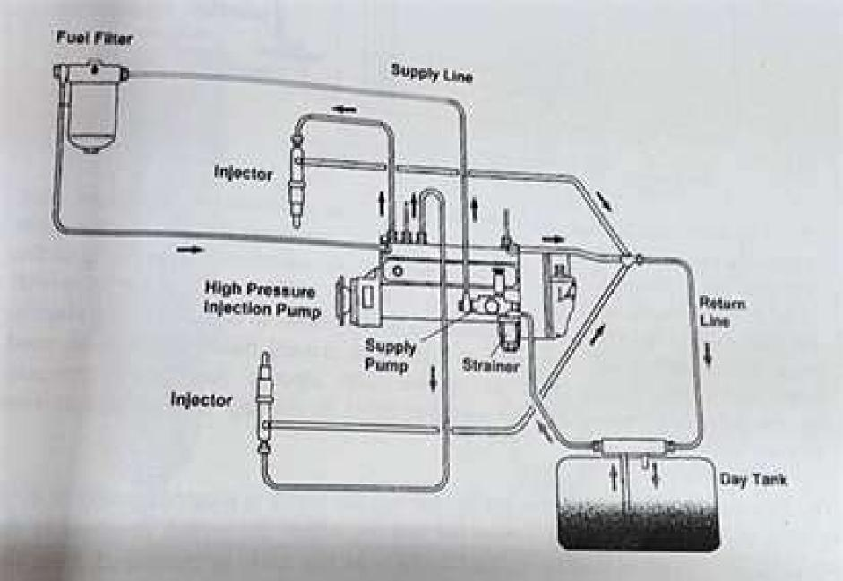
Diesel engine fuel system
