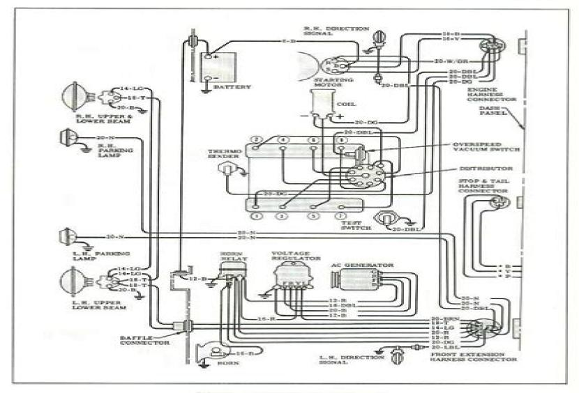
Fig. 39--V-8 Engine Compartment-Model: C-M 80
