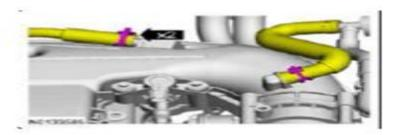
5. Detach the 2 coolant tube retainers from the upper intake manifold.
