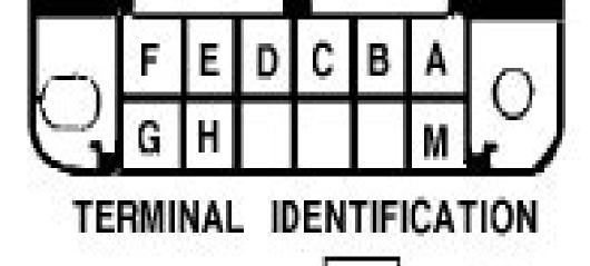
T.C.C. (IF USED) GROUND DIAGNOSTIC TERMINAL FUEL PUMP (IF USED) В G BRAKE SENSE SPEED A.I.R. (IF USED) Н INPUT (CK) SERVICE ENGINE SOON SERIAL DATA (L4) M LAMP (IF USED) (SEE SPECIAL TOOLS) SERIAL DATA E
