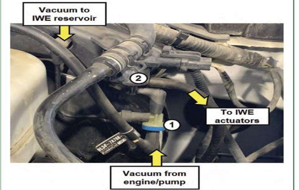
Figure 5: IWE control components are located in front of the brake booster. #1 is the one-way check valve, #2 is the IWE solenoid.
