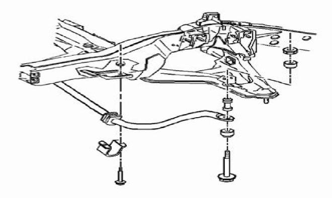
Fig. 4: View Of Stabilizer Shaft Bracket Courtesy of GENERAL MOTORS CORP.
