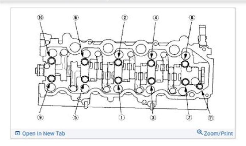
Apply engine oil to the bolt threads and flange. Tighten each bolt two turns at a time in sequence.Specified torque:
