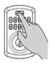
Up to 5 One-time User Codes can be saved. One-time User Codes should be 4 to 8 digits in length. The One-Time User Code will be deleted automatically after it is used. The same One-Time User Code can be created again after it's used.
