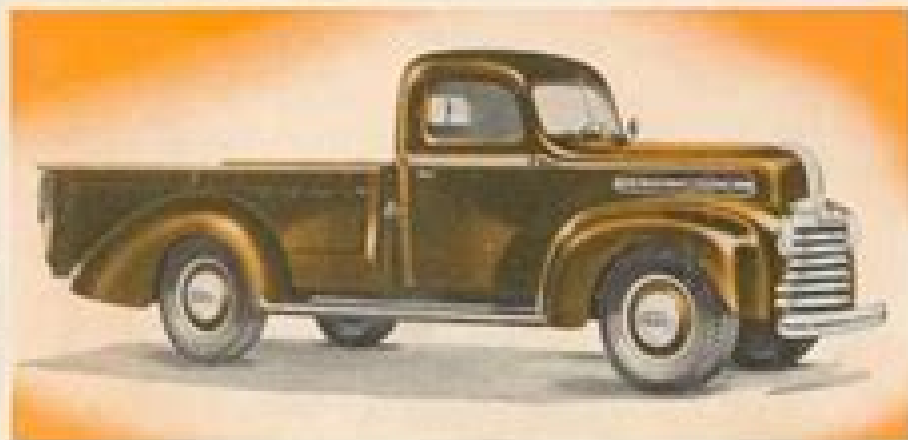
1-TON, 127" W6 EXPRESS. This new Mercury Truck features sturdiness, load space and economy. Heavy-gauge steel body sides. Load length 96.00 inches, width 54 inches, height 22.2 inches. 1.20-17, 8-ply tires are standard.
