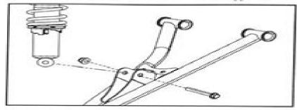
Remove the upper ball joint pinch bolt from the front bearing carrier (see Figure 10-2).
