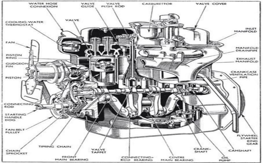
This partly cut-away view of a modern four-cylinder power unit illustrates most of the components. The main features can be quickly identified; the crankshaft which drives the camshaft through a double roller-chain, the pistons, valves and valve gear, the inlet and exhaust systems, and the oil pump which forces oil under pressure through an intricate system of oil-ways in the engine. The only items not shown are the col-ignition distributor and the sparking plugs.
