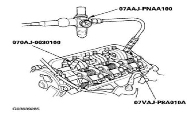
Fig. 7: Installing And Connecting Special Tools (Front) Courtesy of AMERICAN HONDA MOTOR CO., INC.
