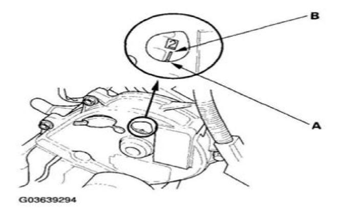
Fig. 16: Aligning Pointer On Front Upper Cover With No. 2 Piston TDC Mark On Front Camshaft Pulley
