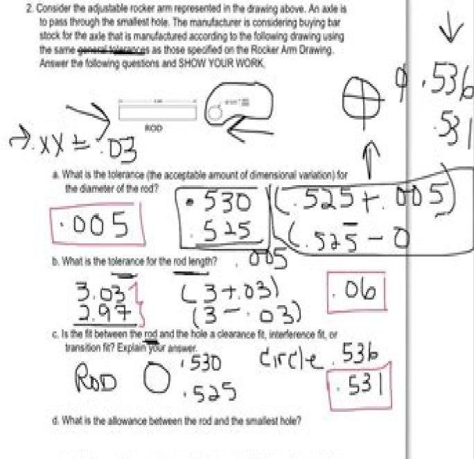
If the design of the assembled machine requires that the rod is sized such that the actual clearance between the rod and the hole is never greater.
