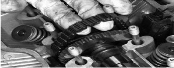
Loop the cam chain over the sprocket.
