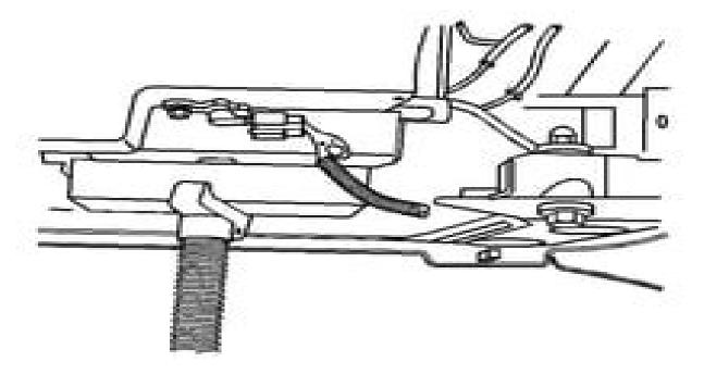
Fig. 2: View Of Wood Block Between Engine Oil Pan & Pole Jack Courtery of GENERAL MOTORS CORP.
