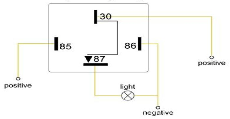
85 and 86 are the relay coil ends, 30 and 87 are the normally open contact terminals of the ralay, when 85 and 86 connect the power, 30 and 87 will be connected.
