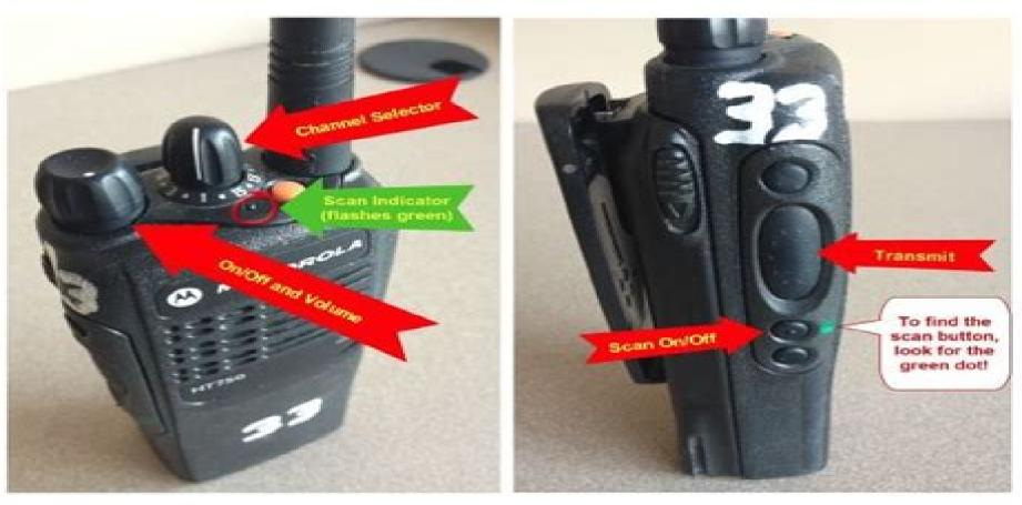
IF you are hearing all the channels, check the SCAN INDICATOR. If it's flashing green, press the scan on/off button to turn scan off (green light will no longer flash)
