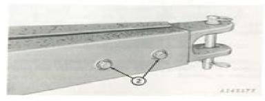
Close hitch and secure with bolts removed in step 5 at left. Tighten to 170 foot-pounds (230 Nm) (230 kgm) torque.
