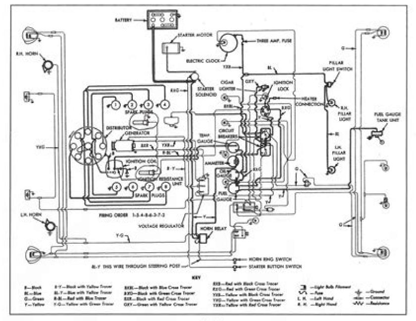
Fig C-4 1947-48 Ford V8 Schematic Wiring Diagram
