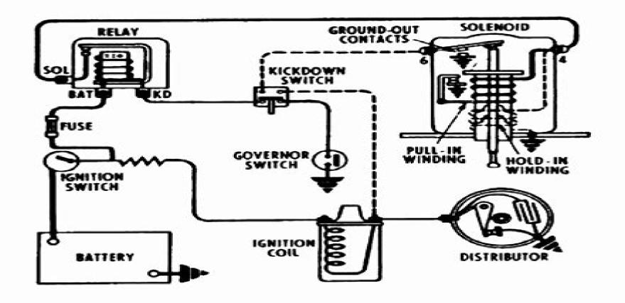
Overdrive Electrical Circuit Wiring Diagram
