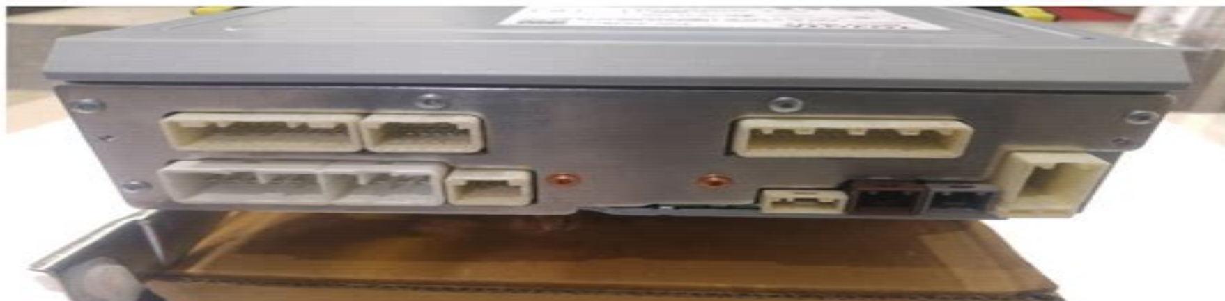
16 pin (10+6) Toyota Head Unit proprietary connector
