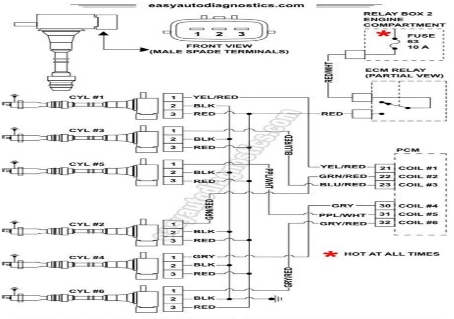
PART 1 -IGNITION SYSTEM WIRING DIAGRAM (2001-2002 3.5L PATHFINDER)
