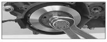
Put the protection cover on the crankshaft thread, twist in the flywheel. extractor and remove the flywheel.
