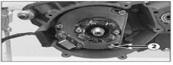
Undo the 3 screws @ and remove the stator together with the base plate.
