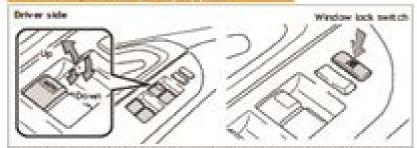
Automatic operation (driver side only) Push the switch completely down and release to fully open. To stop window midway, tightly push the switch in the opposite direction.
