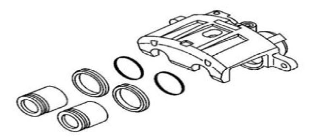
Fig. 8: View Of Brake Caliper Pistons, Boots & Seals Courtesy of GENERAL MOTORS CORP.
