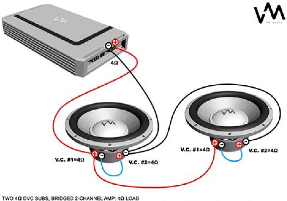
**BRIDGE WIRE** 0 POSITIVE TERMINAL POSITIVE WIRE **NEGATIVE WIRE** IMPEDANCE LEVEL (OHMS) **NEGATIVE TERMINAL**
