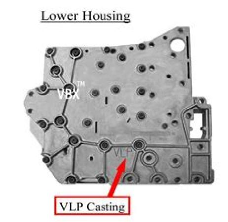
This valve body can be identified by the letters "VLP" cast into both the Upper and Lower Housing (see RED ARROWS), as well as the addition of a pressure sensor (see BLUE ARROW) and pressure solenoid (see GREEN ARROW).
