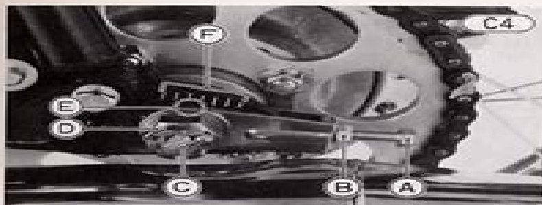
A. Adjusting Bolt B. Locknut C. Cotter Pin D. Axle Nut E. Notch F. Alignment Marks
