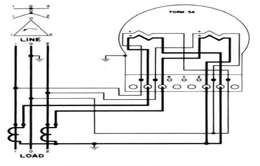
3ø, 3 W OR ANY OTHER 3 W CIRCUIT 2 Stator, 3ø, 3 W Meter with 2-2 W CT's
