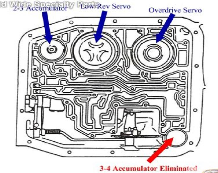
The 3-4 Shift Accumulator used in earlier model AOD transpills in was eliminated in 1989, except on vehicles equipped with
