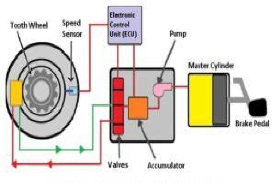
Working of Anti Lock Braking System
