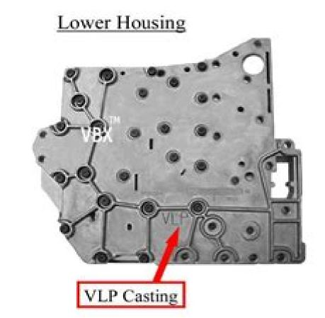
This valve body can be identified by the letters "VLP" cast into both the Upper and Lower Housing (see RED ARROWS), as well as the addition of a pressure sensor (see BLUE ARROW) and pressure solenoid (see GREEN ARROW).
