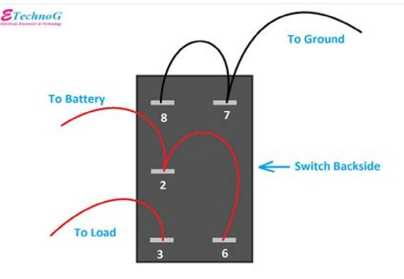
5 Pin Rocker Switch Wiring and Connection Diagram
