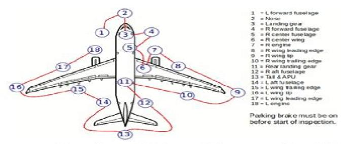
The purpose of the walk-around is to search for any conditions that could compromise the safety of the flight. It is important to perform this task correctly because the consequences of failure can be very serious.
