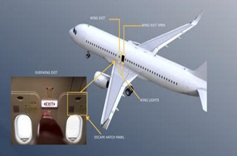
Overwing exits are equipped with emergency exit lighting. An escape hatch handle light, installed above the door frame, will illuminate as with other emergency exit lighting. Exterior overwing exit lights will illuminate the escape path outside the cabin on the wing's upper ourbox. They will illuminate once the overwing escape hatch handle cover is removed.
