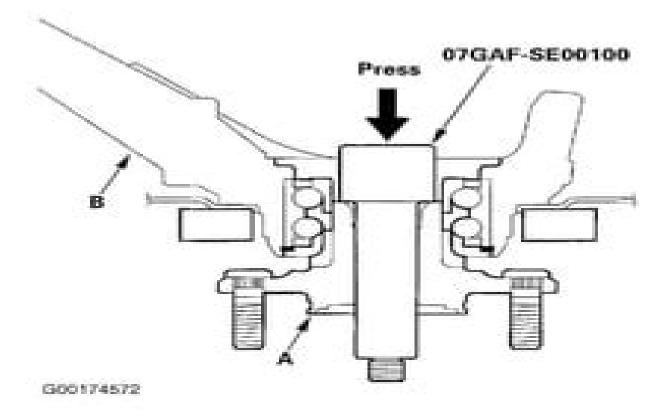
Fig. 12: Separating Hub From Knuckle Courtesy of AMERICAN HONDA MOTOR CO., INC.
