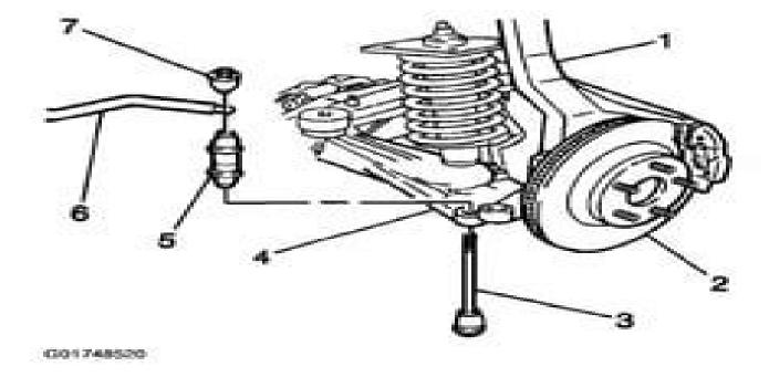
Fig. 5: Installing Stabilizer Shaft Link Courtesy of GENERAL MOTORS CORP.
