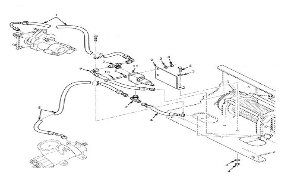
Figure 225K. Hydraulic Winch Pressure Relief Valve Kit and Related Parts (Serial Numbers 246890 and Above).
