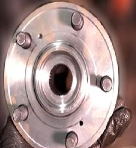
HOW TO REPLACE FRONT WHEEL HUB AND BEARING ASSEMBLY 2007-2013 ACURA MDX
