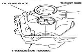
8. Remove the 10 mm sealing bolt and oil gutter plate.
