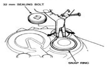
Expand the snap ring on the countershaft ball bearing and remove it from the groove using a pair of snap ring piler.
