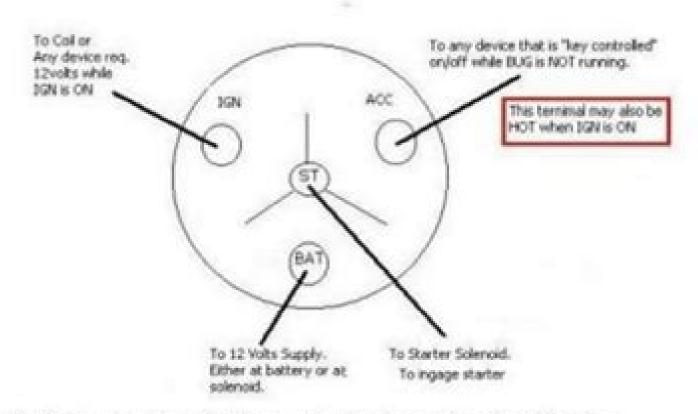
Back, side of generic ignition switch. It does not matter where the terminals are physically located on back of switch. What matters is that the designation of the terminal, matches the function one is trying to use it for.
