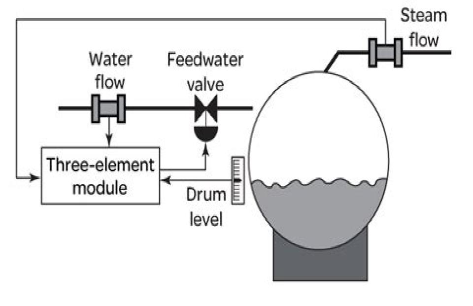
Figure 3 Three-element drum level control
