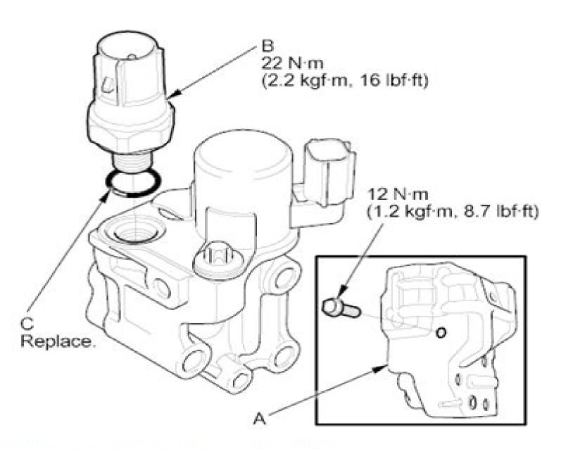
Remove the rocker arm oil pressure switch (B).
