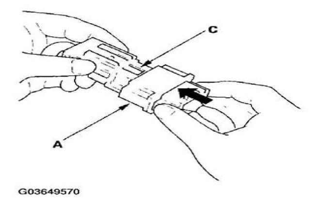
Fig. 16: Holding Pawl-Side Connector And Pressing On Back Of Sleeve-Side Connector Courtesy of AMERICAN HONDA MOTOR CO., INC.
