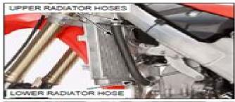
Remove the bolt, ground wire and connector stay boss from the right side radiator lower mount.
