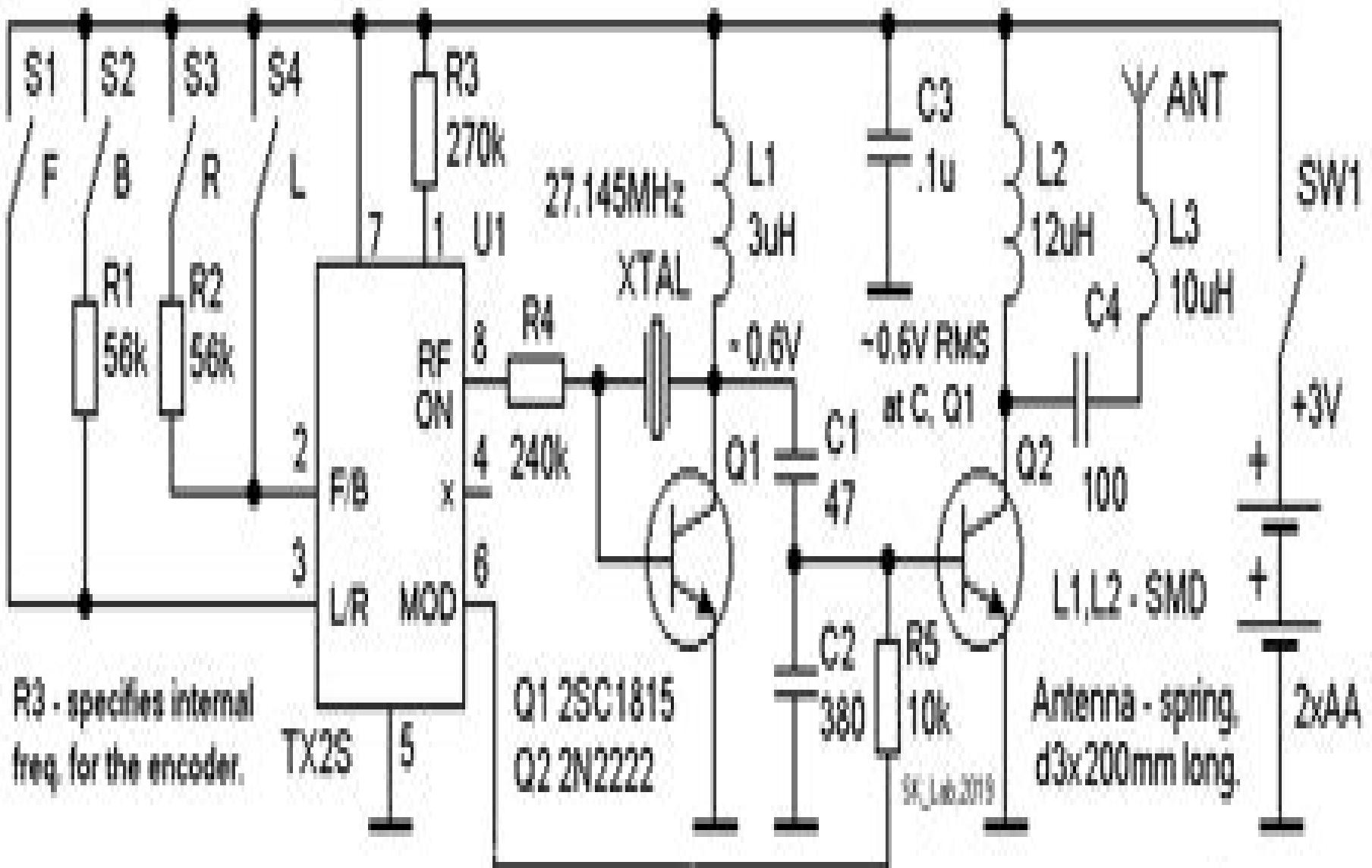
The simplest AM transmitter (27MHz) for a radio controlled toy. Works as it is, and does not require any tuning or so.
