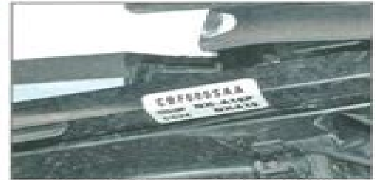
The colour code label is on the rear sub-frame
