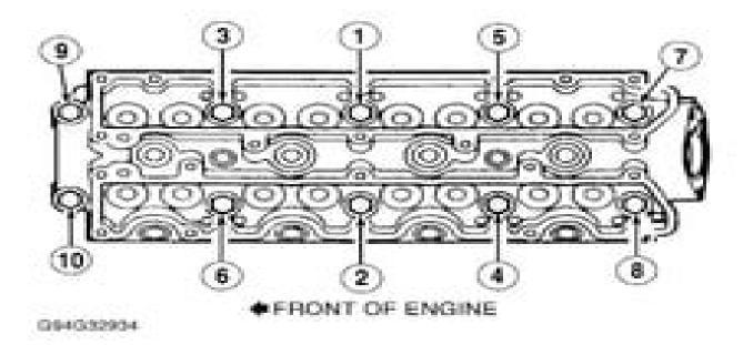
Fig. 4: Cylinder Head Bolt Tightening Sequence Courtesy of GENERAL MOTORS CORP.
