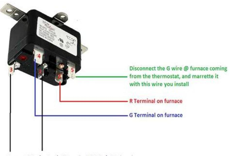
Connect #3 wire to pin #5 on the HRV 9-pin Molex plug and the #1 wire to pin #7
